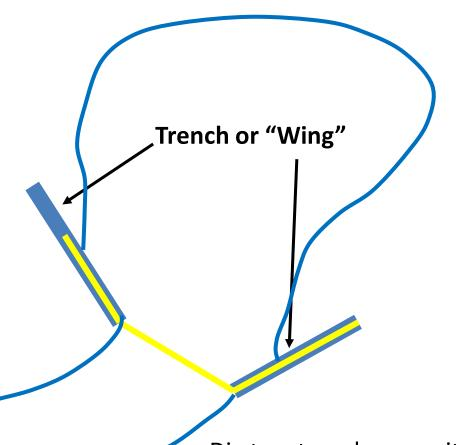
Dig two trenches on either side of the spring to be filled with cement. The "wings" will serve to capture groundwater into the spring box
