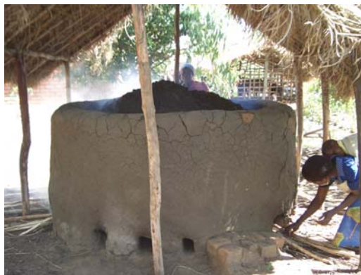
Photo (vb): Mkwaila – kiln firing
