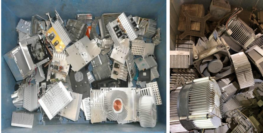
Figure 20: Aluminium fraction from flat panel screens
