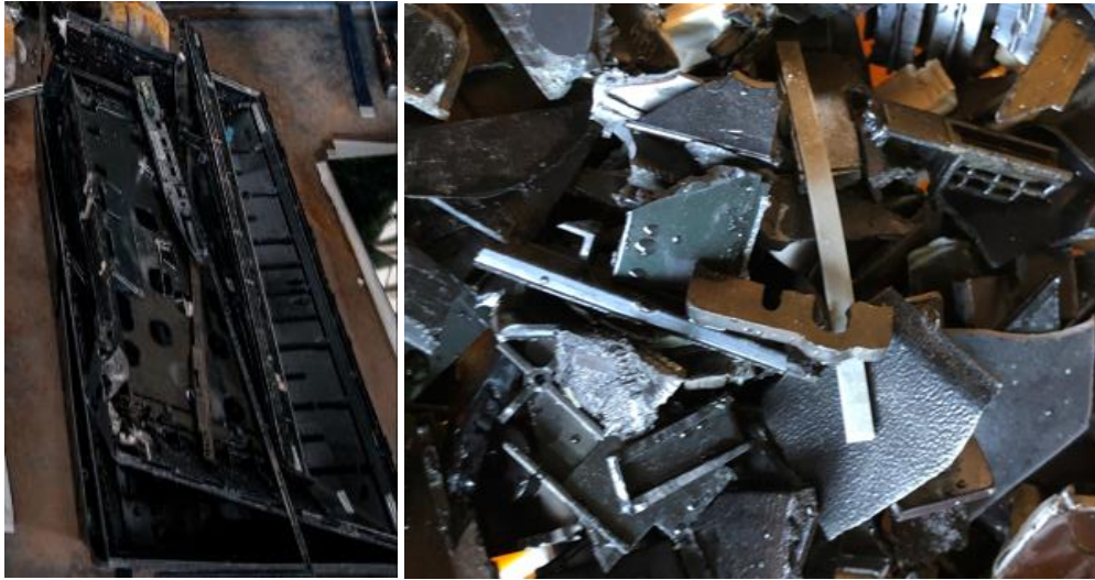
Figure 18: Samples of ABS plastic fractions containing brominated flame retardants (BFR)
