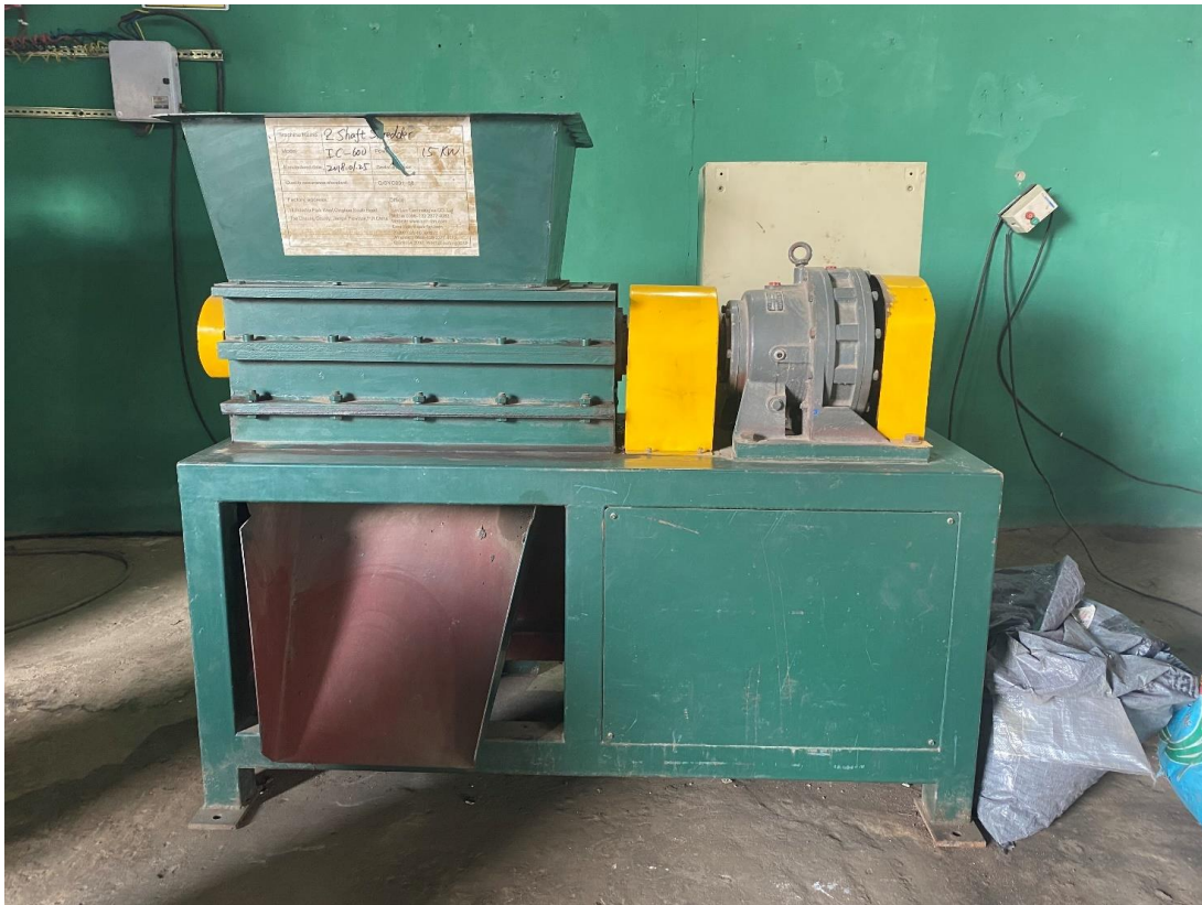
Figure 17: Mechanical shredder for de-polluted and sorted e-waste plastics
