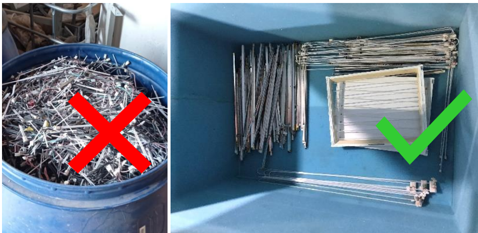
Figure 8: Unsafe storage of broken (!) mercury lamps (left) compared to handling with due care (right)
