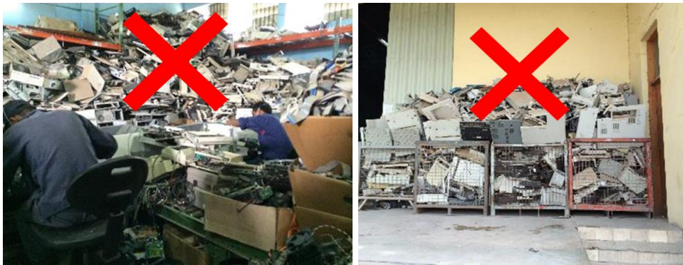
Figure 7: Careless storage and overcrowding of crates with e-waste fractions
