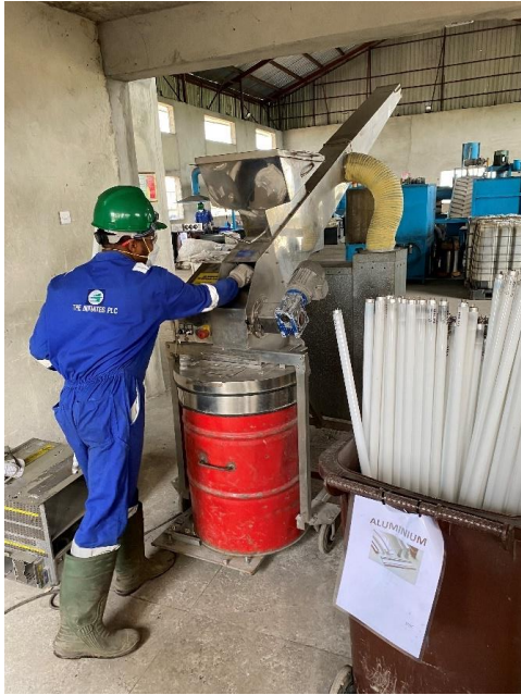
Figure 16: Filtering of mercury lamps in a 'bulb-eater'
