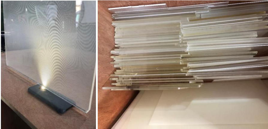
Figure 22: Polymethyl methacrylate (PMMA) layers in flat panel displays
