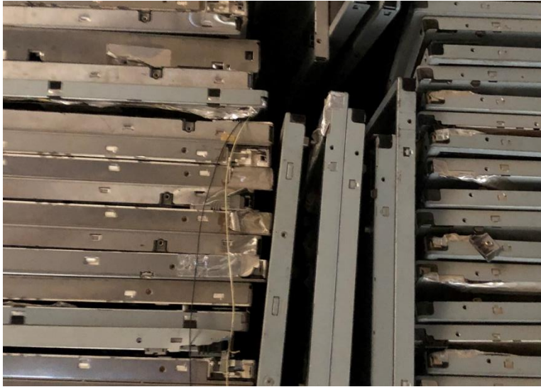
Figure 10: Intact display units for re-use in new televisions.
