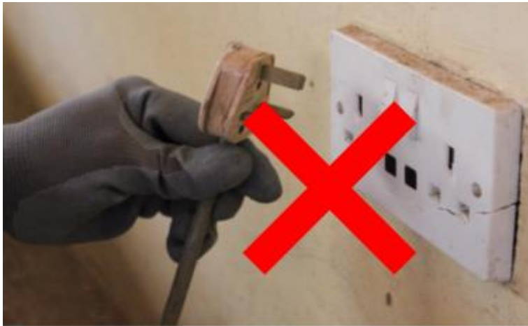
Figure 9: No re-use screening via plug-in and function test
