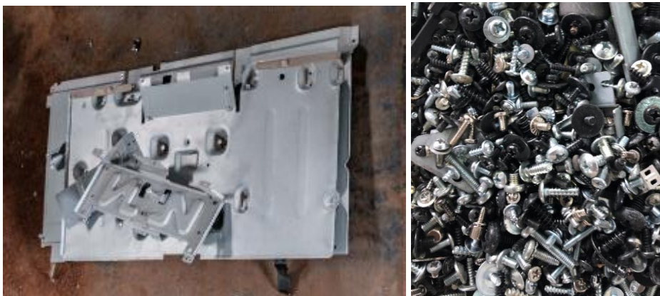
Figure 19: Ferrous metal fraction from dismantled flat panel screen
