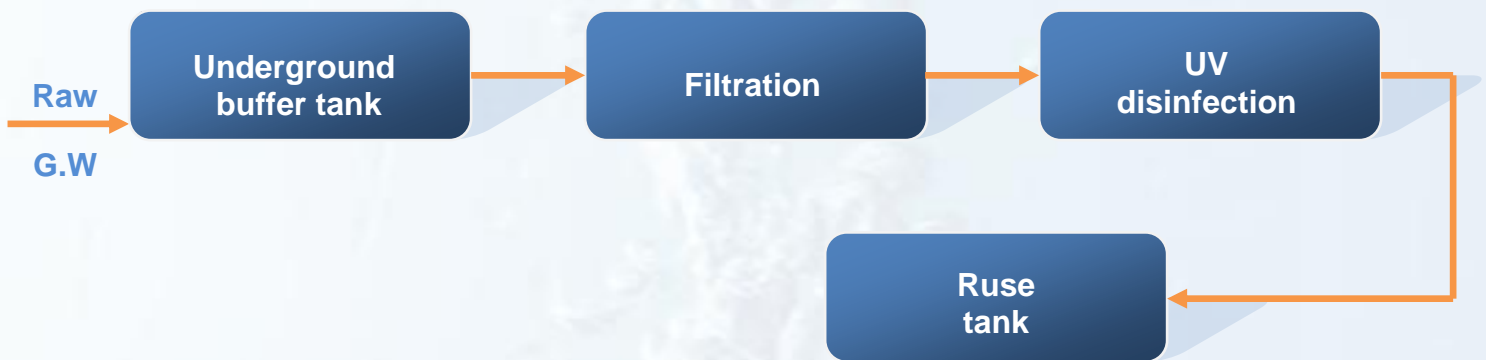
Fig. 4.35: Simple block flow diagram for Aqua reuses domestic GWTS
