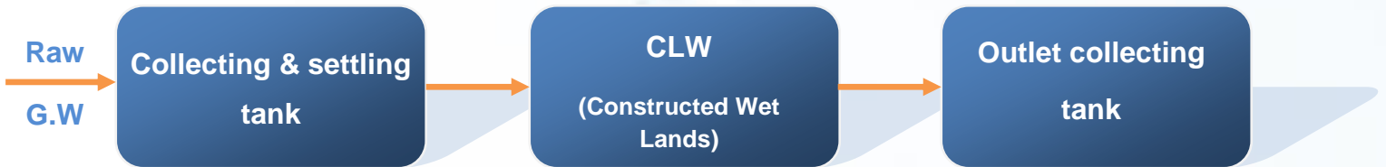
Fig. 4.37: Simple block flow diagram for Constructed Wet Lands CWL
