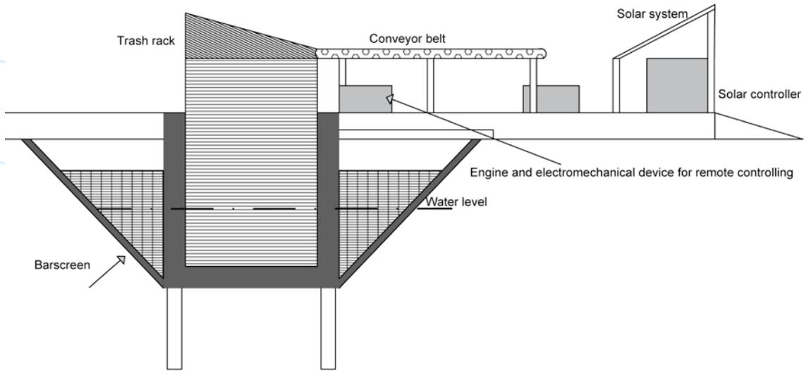
Figure 23: Back view of automated trash rack structure with continuous travelling screen, 2020
