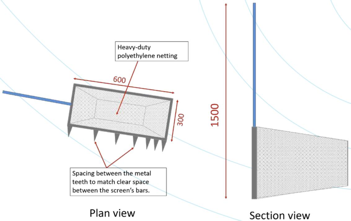
When used in combination, the working platform and the manual rake help address the challenges currently experienced during the operation of the bar screen. However, a significant labour force input is still required. With the aim of providing a complementary solution that reduces human labour force input and that enables a quicker and more efficient cleaning of the bar screen, additional design features have been developed.
