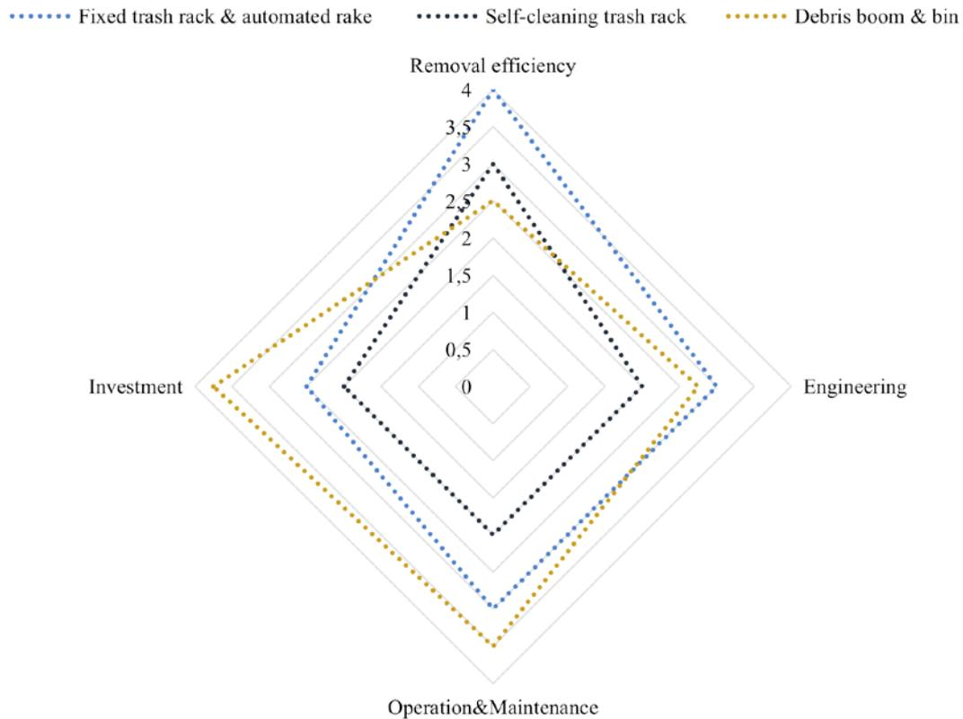
Figure 46: Comparison of upstream sediment control structures, 2020
