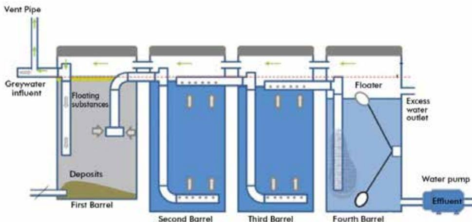
Figure 22. 4-Barrel System setup, for up a family of 6 (Ghougassian, 2013)
