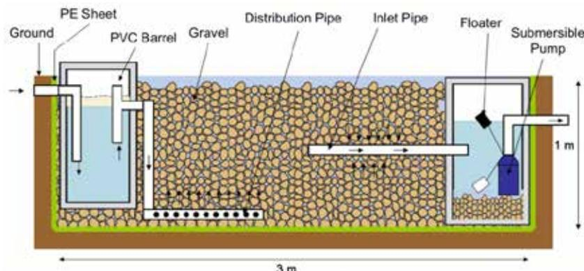
Figure 23. Confined Trench setup for maximum 10 people (Ghougassian, 2013)
