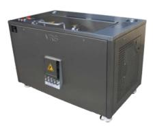
Figure 14. The VRS system has a treatment capacity of 150 kg/day. (Source: Value Recovering Systems Inc.) The VRS system, developed by Value Recovery Systems Inc., relies on a dehydration process. The process involves grinding, water evaporation and the sterilisation of the organic wet waste.
