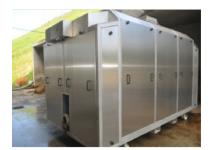
**Figure 16.** The RMO system has an average treatment capacity of three tons/day. (Source: Christophe Grange)
