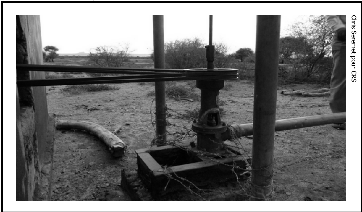
A screw pump operated by drive belts turned by a diesel engine in Tanzania.
