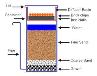
Cross-Section of Kanchan<sup>™</sup> Arsenic Filter
