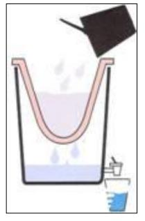
Cross Section of Ceramic Pot Filter (Credit: Filter Pure Inc)
