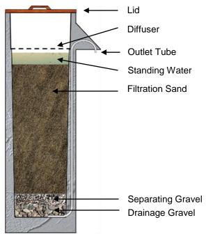
Cross-Section of Concrete Biosand Filter
