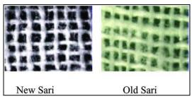
Electron micrographs of a single layer of sari cloth filters (Credit: Colwell et al., 2002)
