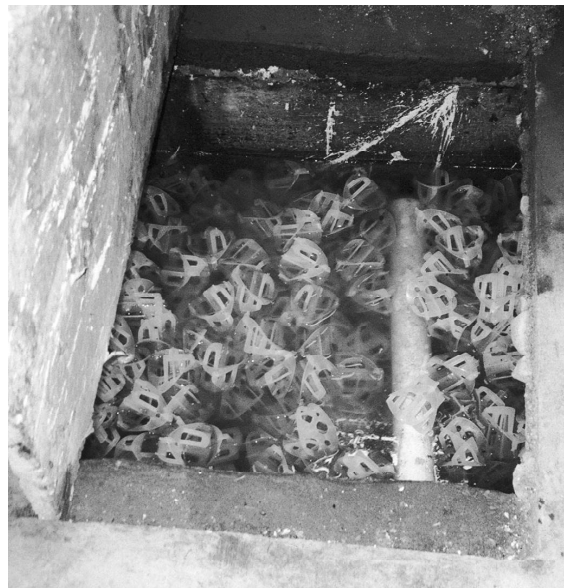
Fig. 21. Floating filter balls made of plastic. When bacteria film becomes too heavy, the balls turn over and discharge their load. The filter medium has successfully been used for tofu wastewater by HRIIE in Zhejiang Province/China. [photo: Sasse]
