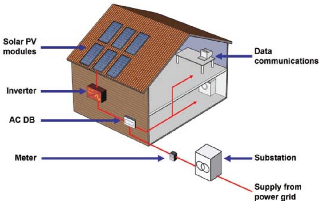
**Figure 2. Grid-connected solar PV system configuration**
