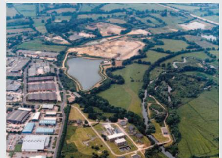
**Top** Little Testwood Lake, one of three disused gravel pits, is now a reservoir with a storage capacity of 270m litres. **Left** Two of the lakes have been converted in to nature conservation areas, benefitting the 200,000 inhabitants in and around Southampton. **Right** Little Testwood Lake is 800m away from the River Test, the previous source of raw water.
