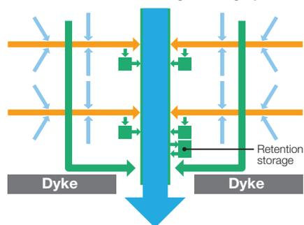
Ho Chi Minh City's drainage system has two different modes of operation requiring different improvement strategies: (a) divert discharge of stormwater in to the Saigon and Dong Nai Rivers and (b) at high tide or times of storm surge, gates closed to retain water within the catchment. Arup's recommendations were (c) adding retention storage along the canal system and a diversion system so that stormwater bypasses flood prone areas.
