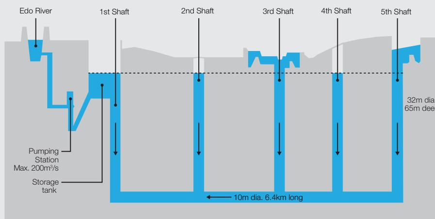
The hydraulic stormwater tunnel system discharges floodwater to the downstream underground storage tank. The pumping station which is located adjacent to the storage tank pumps floodwater at a maximum rate of 200m³/sec to the Edo River.
