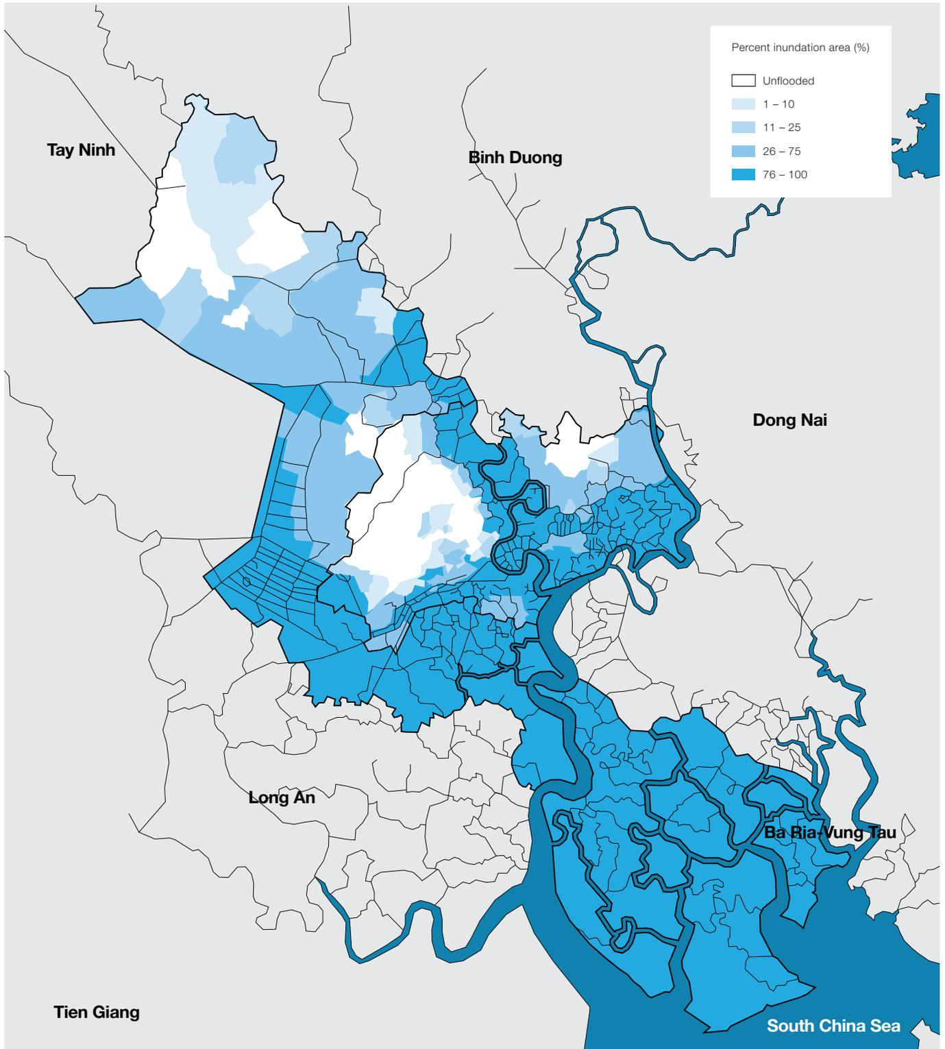
Ho Chi Minh City's vulnerability to urban flooding: the above map, extracted from the ICEM report 'Adaptation to Climate Change', shows the % area of HCMC that will be affected by flooding under combined heavy rainfall, high tides and wind and storm surge typical of a '30-year' storm, e.g. Tropical Storm Linda in 1997. Almost the entire city would be severely affected by flooding.
