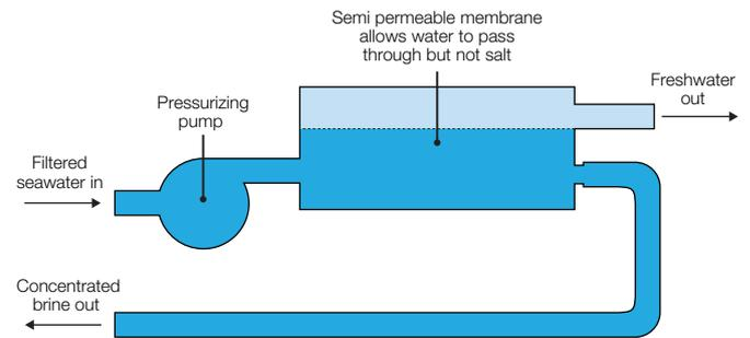
The RO treatment process works by forcing water under pressure through a membrane. The membrane is specifically designed so that the salt fraction and other impurities in the water stream do not pass through and the concentrated brine solution is held and discharged to waste from the upstream side of the membrane. In hotter climates the brine waste is evaporated in ponds so that the residue with value can be disposed of more readily.
