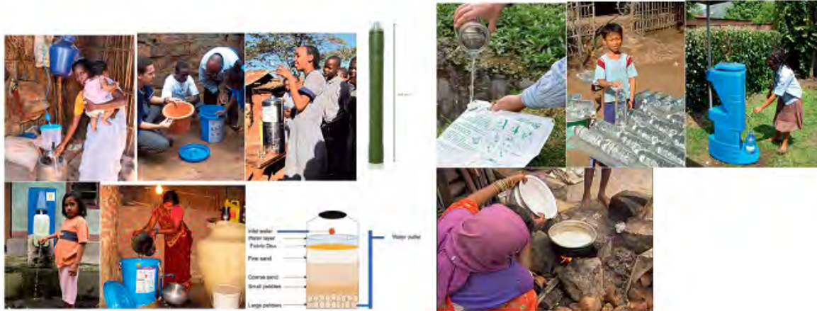
Physical filtering: clock wise from top left: Tulip, Ceramic Pot Filter, Water for Life candle filter, slowsand filter, Kanchan filter and biosand filter
