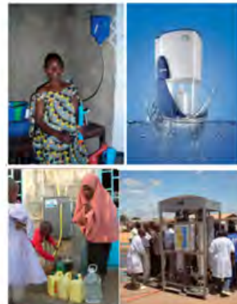
Physical inactivation: clock wise from top left: Aquapack (solar heat+UV), SODIS, Naiade (solar driven UV-lamp) and boiling
