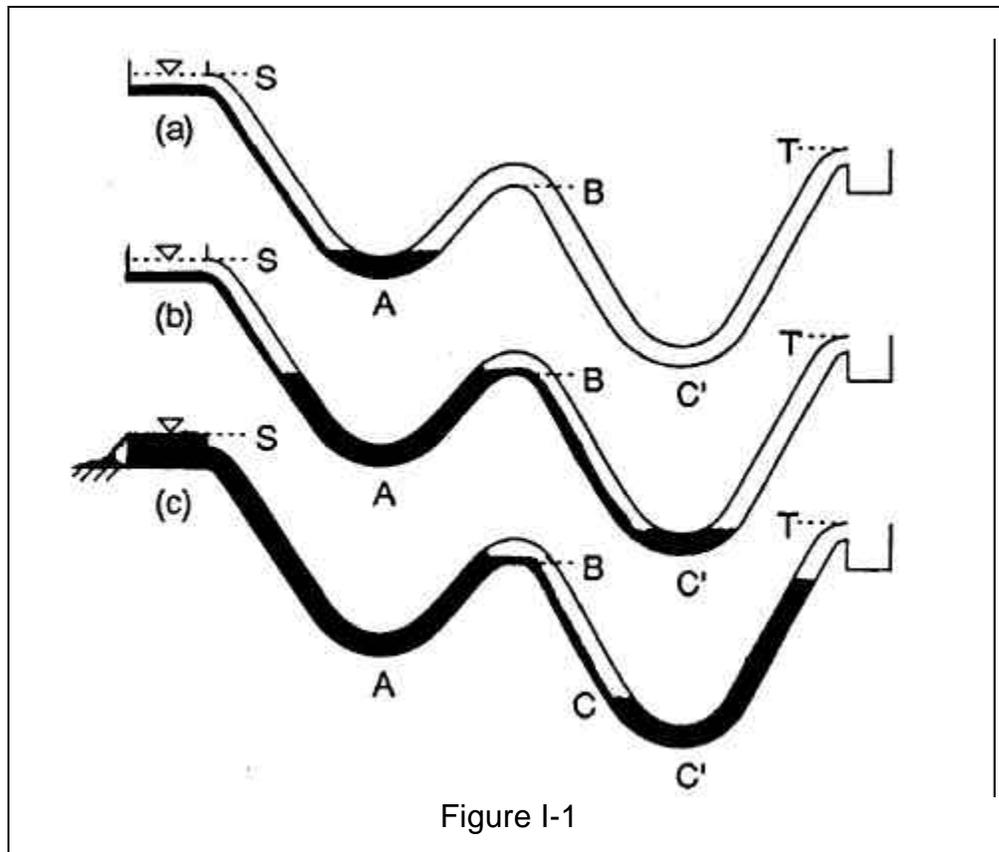
first time a newly constructed gravity flow pipeline since this pipeline starts out at least partially full of air. If, as in figure I-1, the profile has a local maximum (point B) between spring S and tank T, as you allow a small flow of water out of S, the water will accumulate at the low point A and then, fill the pipe on both sides of A
