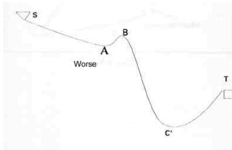
3) **Between two equally high high points followed by low point of unequal heights, choose the one with the higher low point.**
