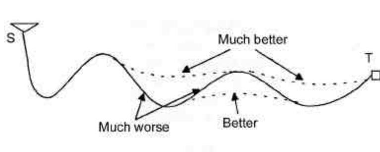
4) Finally- and this one is frequently an effective option, **for two high points of equal height followed by two low points of identical height, choose the one for which the trench profile maintains its height longest and drops down to the low point latest.** The effect of this simple option is especially large when the pressure at the high point is substantially larger than atmospheric.
