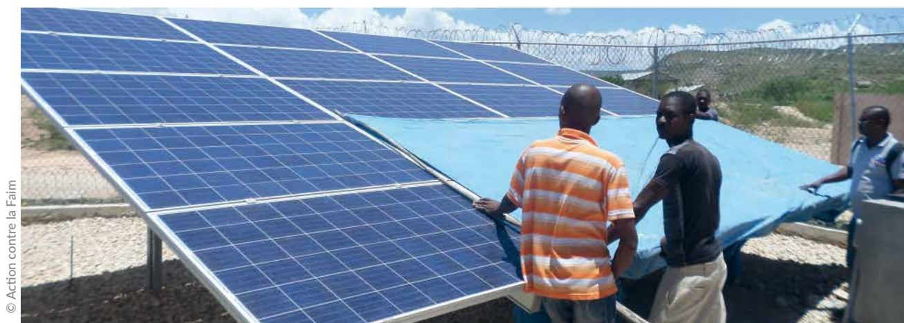
Tarpaulin test for partial covering to verify that the pump adapts its power depending on sun power.
