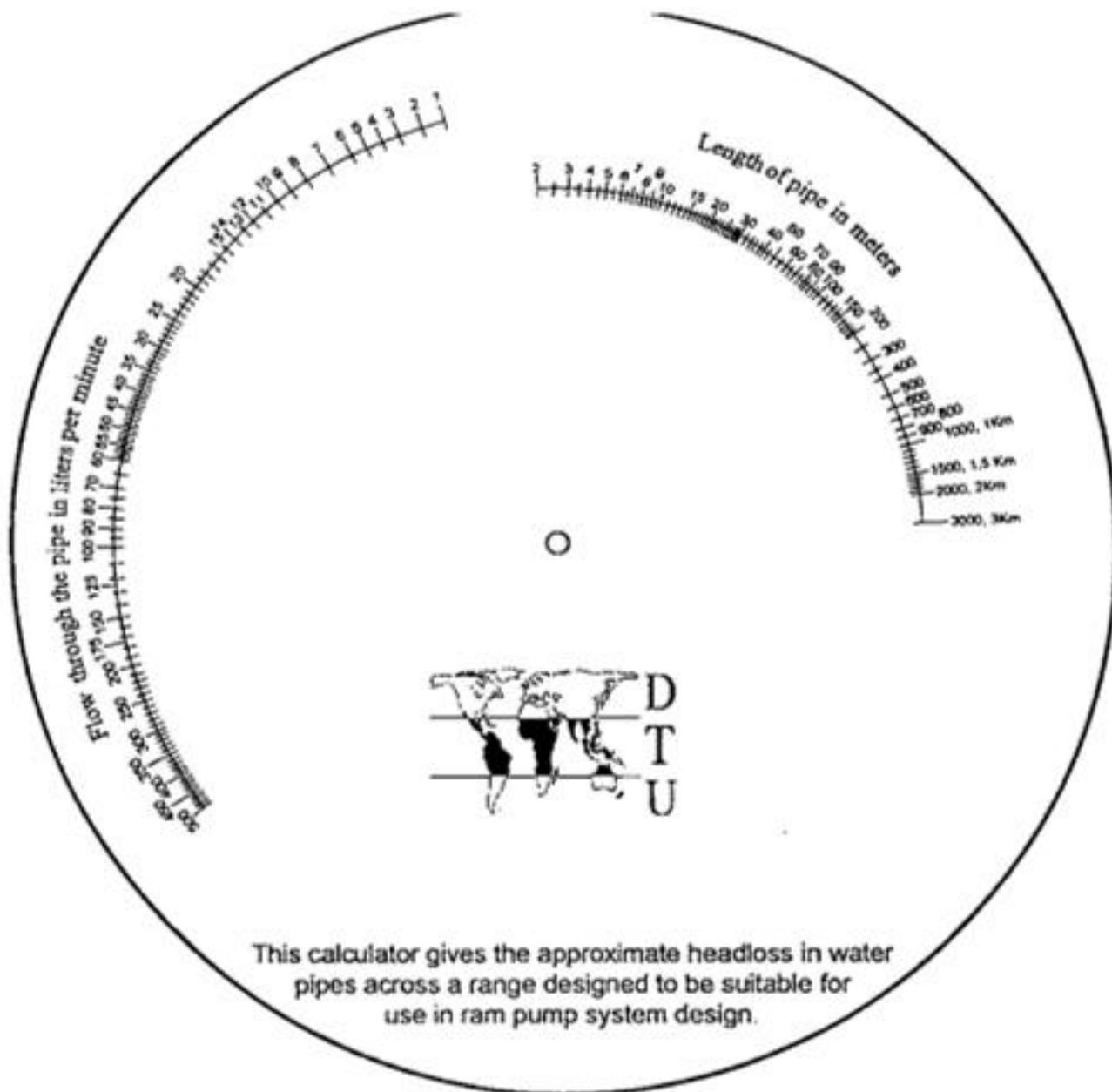
This calculator gives the approximate headloss in water pipes across a range designed to be suitable for use in ram pump system design.
