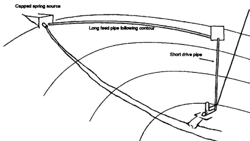
Figure 18: Topography and drive pipe position
