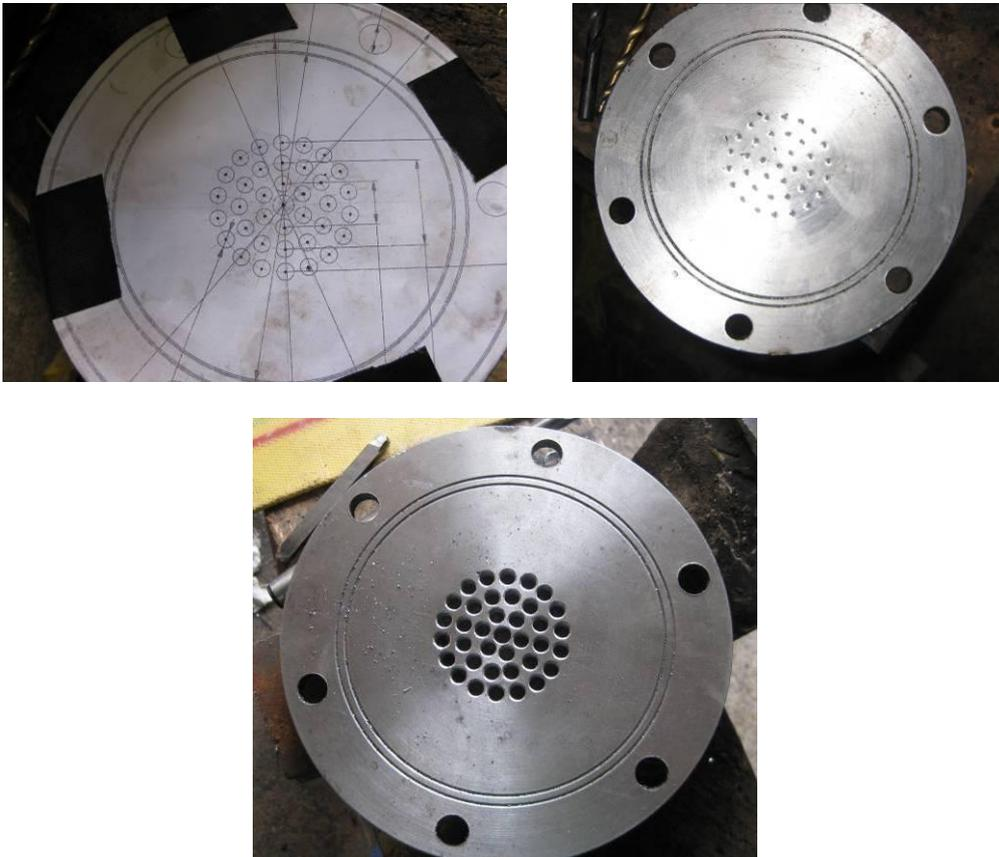
Figure 33: Delivery valve manufacture
