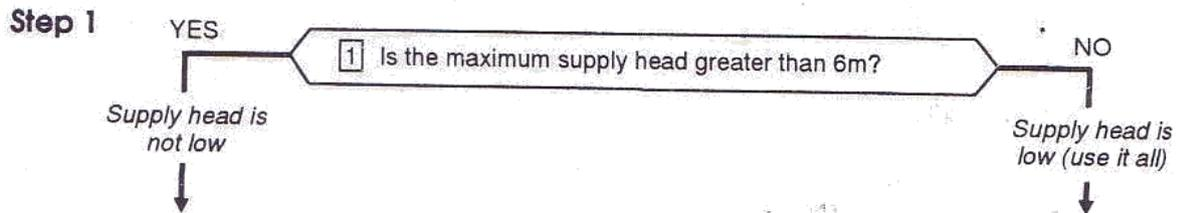
In situations where the drive head is quite low (under 6m) the maximum drive head available ( $H_{max}$ ) should be used. Where the drive head available is greater than 6m, a balance between drive head and drive flow must be found in order to give the required delivery flow.
