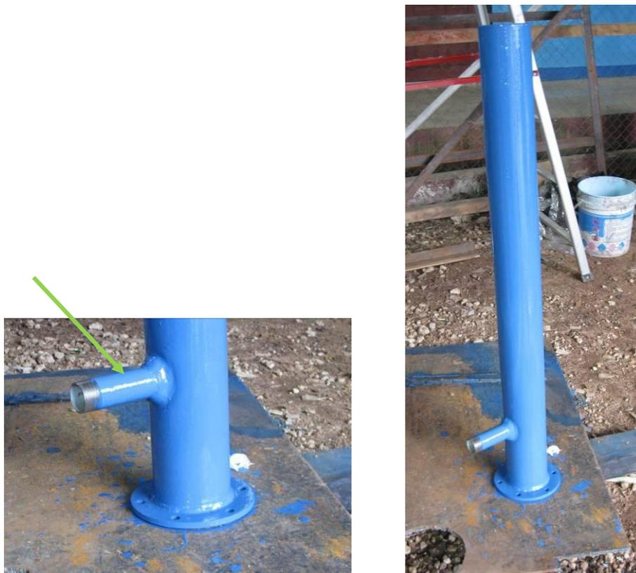
Figure 15: Air vessel
