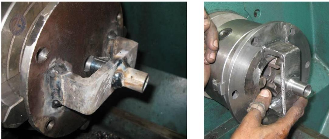
Figure 35: Manufacture of the top of the impulse valve plate
