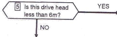
The maximum supply head ( $H_{max}$ ) of this site is greater than 6m (Step 1). Under these circumstances the drive head to be used should be at least 6m. If the drive head calculated in Step 4 is less than 6m, the head to be used should be set at 6m and the number of pumps and the drive flow required recalculated. (Steps 10 to 12.)
