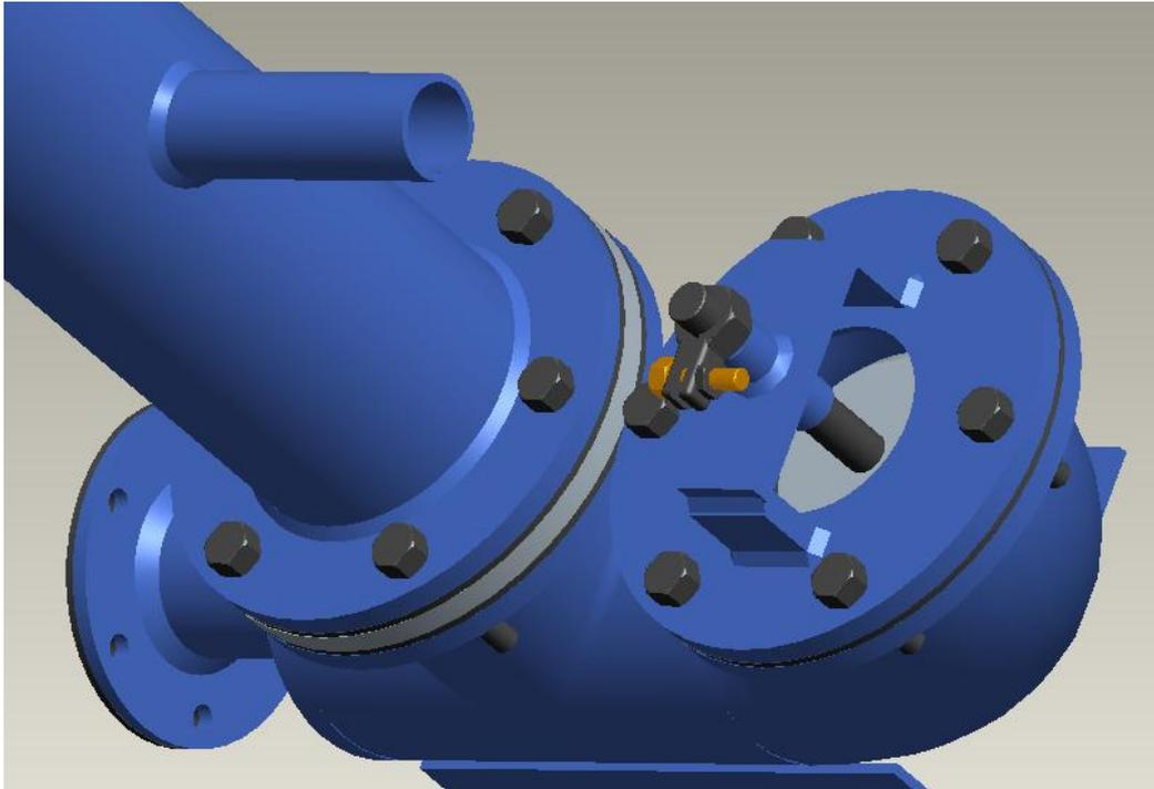
Figure 11: Hydraulic Ram Pump from ACF design
