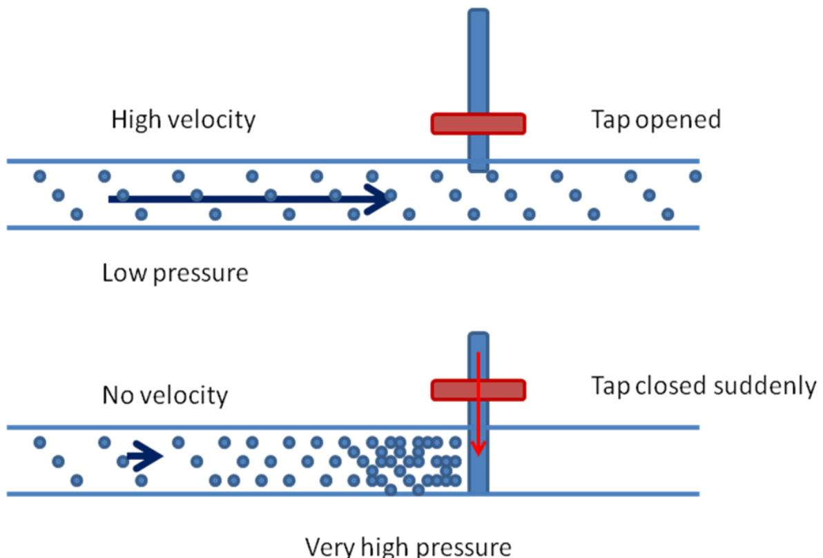
Figure 2: Water hammer effect
