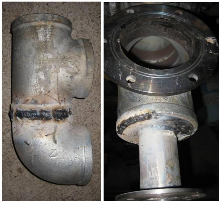
Figure 30: Welding the pump body
