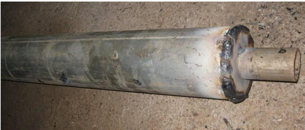
Figure 38: Manufacture of the air vessel
