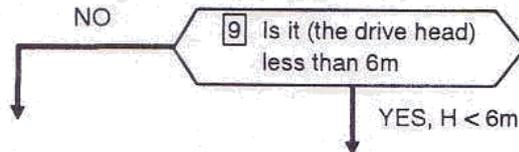
The maximum supply head ( $H_{\max}$ ) of this site is greater than 6m (from Step 1). If the drive head calculated in Step 8 is less than the minimum value of 6m, it should be increased (Step 10).
