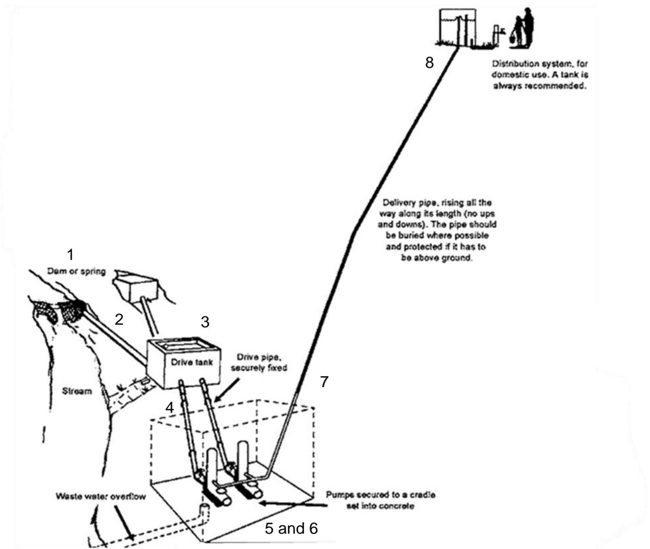
Figure 4: Hydraulic Ram Pump System
