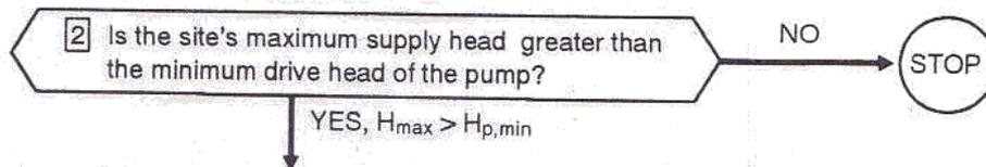
If only a very small supply head is available ( $H_{max}$ ), check that it is larger than the minimum ( $H_{p,min}$ ) from which the pump can operate with a reasonable output. If the available head is too low it may be possible to select a different pump that is capable of using the low head, but a site with a higher head will probably be required.
