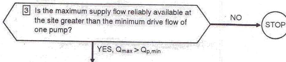
Check that the maximum supply flow available ( $Q_{max}$ ) at the site is greater than the minimum drive flow ( $Q_{p,min}$ ) required by one pump. If there is not enough water to run the pump, a smaller pump may be used, or a site with a greater supply flow must be found.
