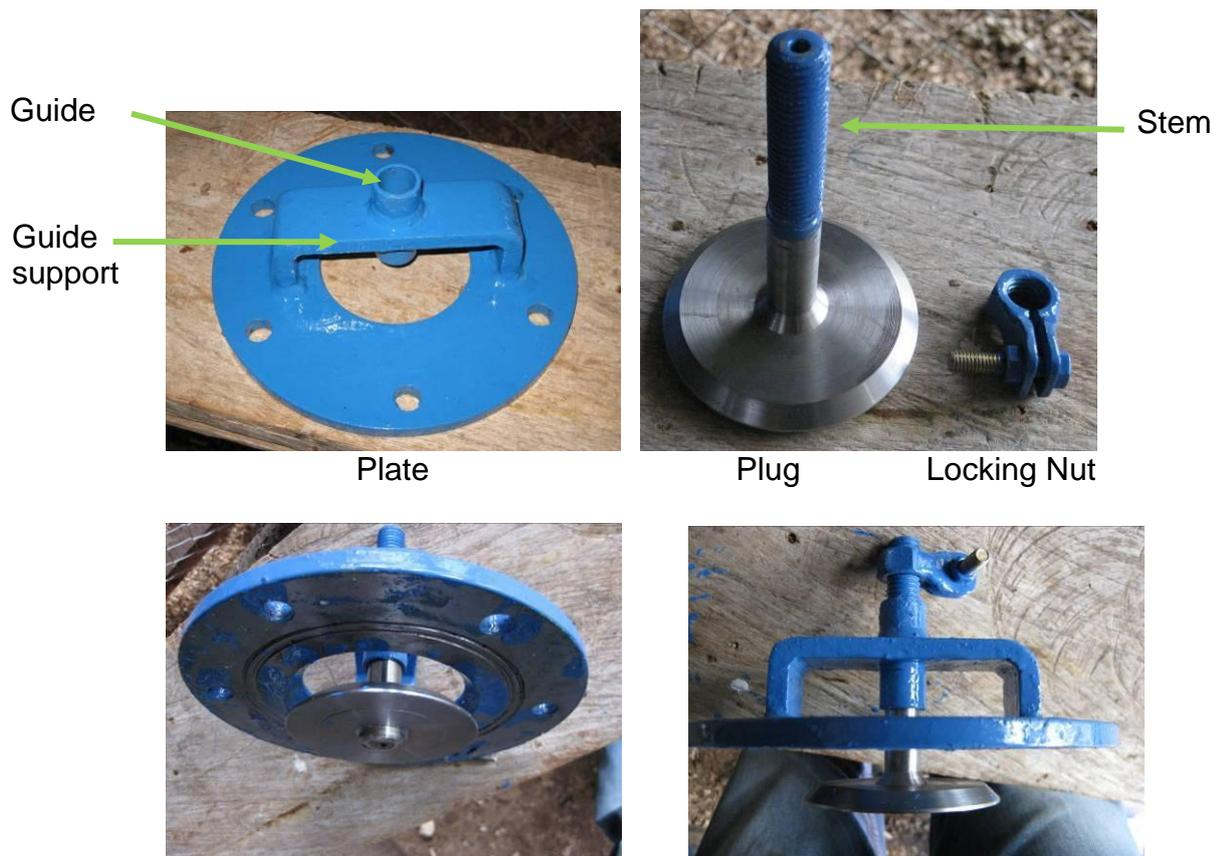
Figure 13: Impulse valve and its components
