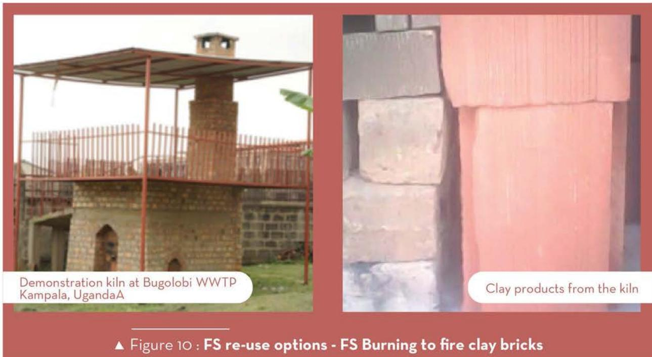
▲ Figure 10 : FS re-use options - FS Burning to fire clay bricks
