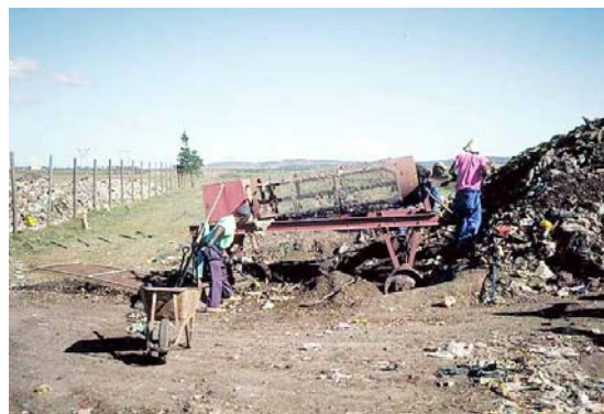
Figure 3-2 Sieving of matured compost in a rotary sieve at the Rini/Grahamstown (South Africa) co-composting works
