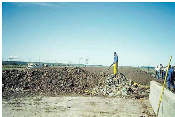
Figure 3-1 Sprinkling FS over refuse at the Rini/ Grahamstown (South-Africa) co-composting plant
