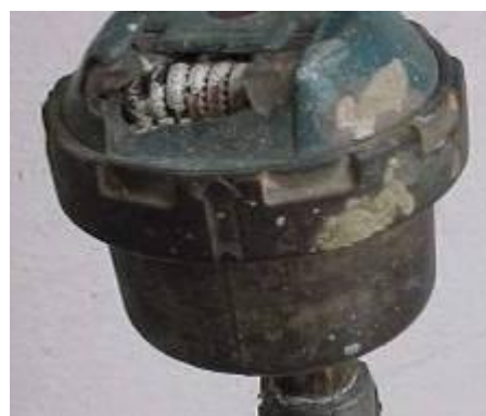
The customer has tampered with the meter's moving parts.
