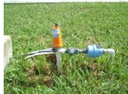
Noise loggers can be deployed on fittings in the network.
