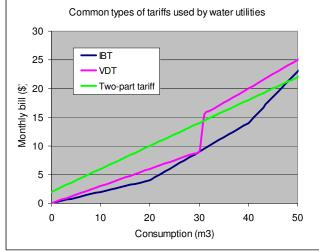
Figure 2 : Shape of Common Types of Tariffs Used by Utilities as a Function of Consumption
