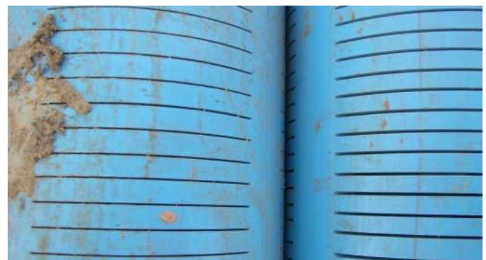
Figure 4: PVC screen (left 0.75mm slot, right 1mm slot)
