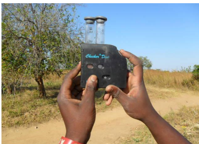
Figure 10: Checking iron content at the wellhead
