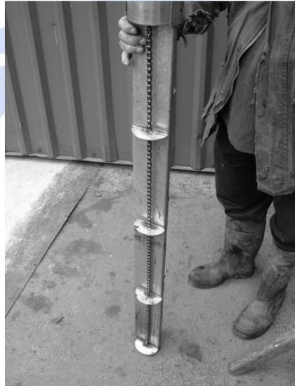
Figure 2 Continuous chain device [Sugden, 2008]
