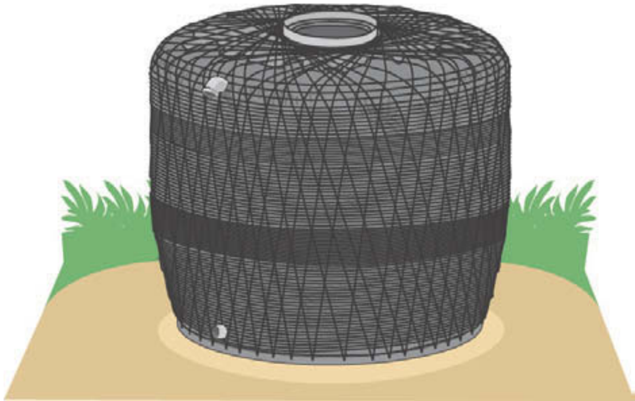
Fig. 37: Jar after completion of horizontal wire wrapping
