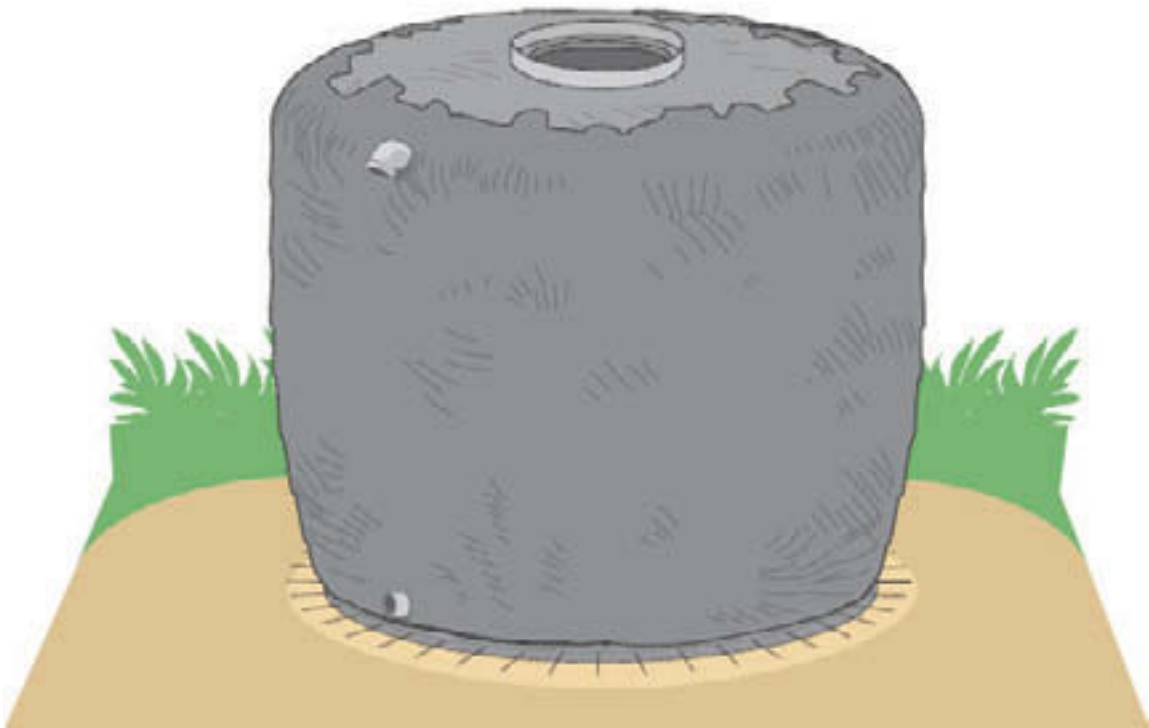
Fig. 31: Second coat of cement mortar
