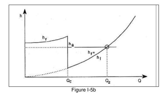
If as in Figure I-5b, the horizontal line  $h_a$  is lower than  $h_r$  even at Q = 0, water will not flow at all **unless enough air is first bled out of the socks so that the curve**  $h_r$  falls below  $h_a$ . If you do bleed the air, you will be able to have a supercritical flow up to  $Q_2$ , provided of course that the spring output is sufficient.
