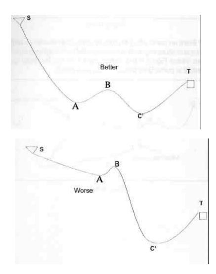
3) Between two equally high high points followed by low point of unequal heights, choose the one with the higher low point.
