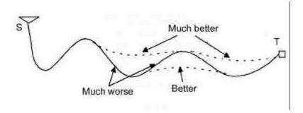
4) Finally- and this one is frequently an effective option, for two high points of equal height followed by two low points of identical height, choose the one for which the trench profile maintains its height longest and drops down to the low point latest. The effect of this simple option is especially large when the pressure at the high point is substantially larger than atmospheric.
