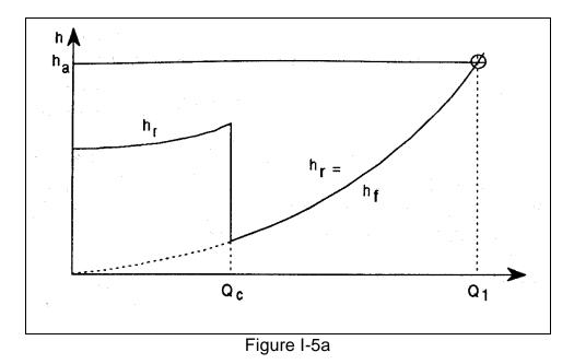
The smallest value of Q for which this line crosses the head required curve is the maximum flow rate, which the pipeline can deliver. If as in Figure I-5a, the horizontal line  $h_a$  lies above the curve  $h_r$  for low values of Q, and crosses it only once, the situation is simple: the pipeline will accommodate the flow rate of the spring from Q = 0 to  $Q_1$ , the crossing point, and if the spring output is larger than  $Q_1$  the excess will spill at the spring.
