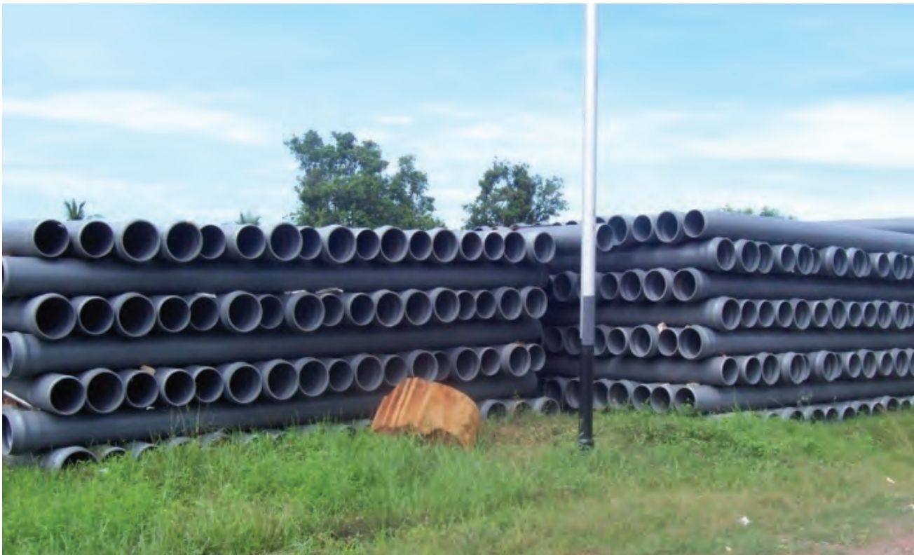
High-density polyethylene pipes for transmission mains
